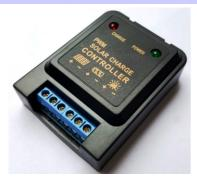
This unit is an electronic switch that switches on the connection to the solar cells if the battery is empty and switches off again when the battery is fully charged. There is a charging LED and a battery full LED on the unit.
